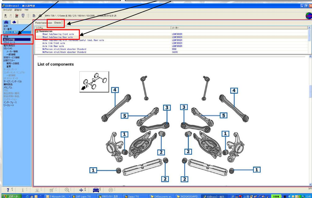
The screenshot shows the ESI[tronic] software interface. The left sidebar contains a navigation menu with '組立説明書' (Assembly Manual) highlighted. The main window displays a tree view of components, with 'Suspension' selected under 'Chassis'. Below the tree view, a 'List of components' section shows a detailed diagram of the suspension assembly with numbered callouts (1-5) pointing to various parts.
