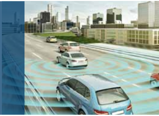
Lane change assist warns drivers if there are vehicles in an area critical to changing lanes.
