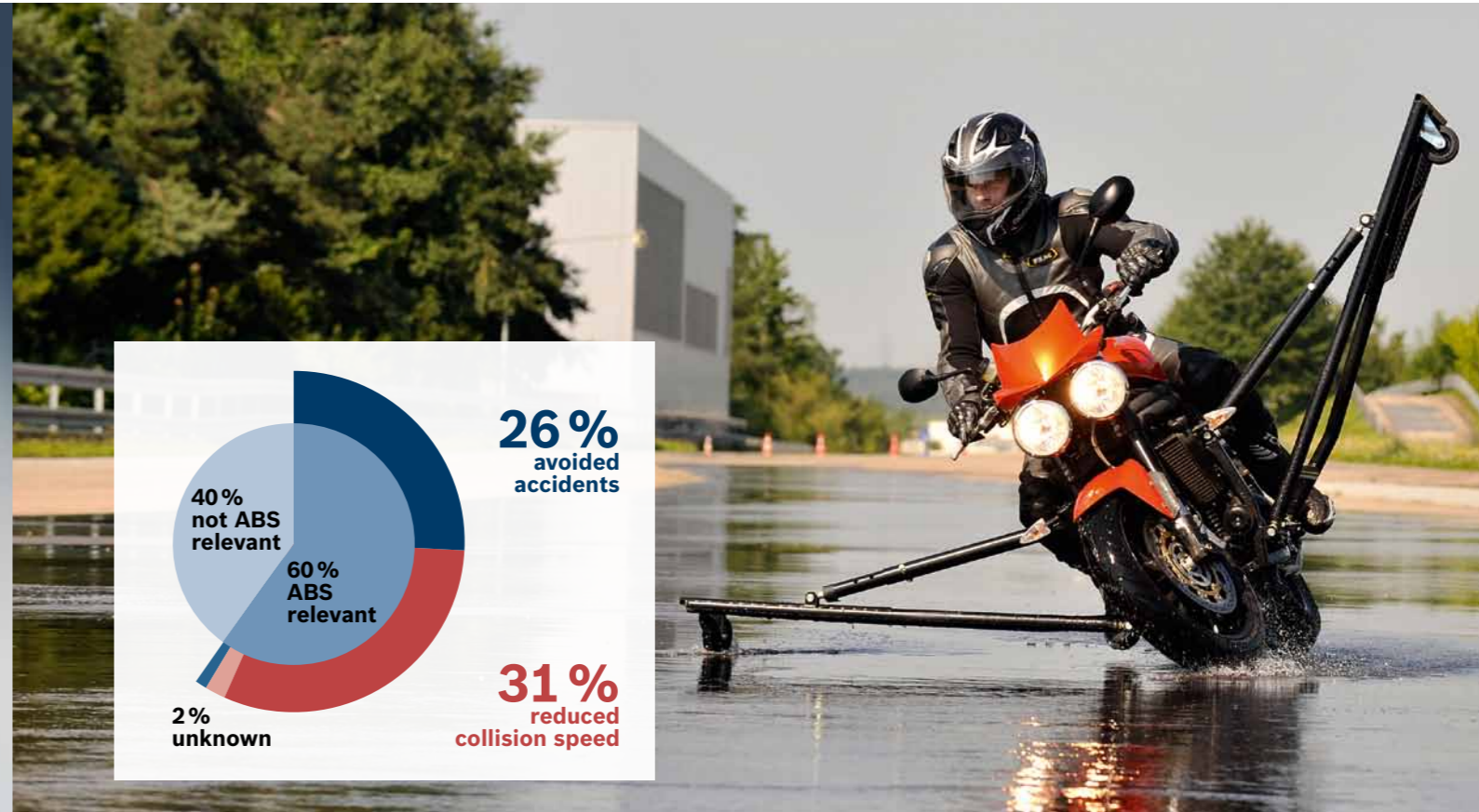
Bosch ABS benefit study based on GIDAS (German In-Depth Accident Study, 2001-2009) powered two-wheelers involved in accidents with injuries
