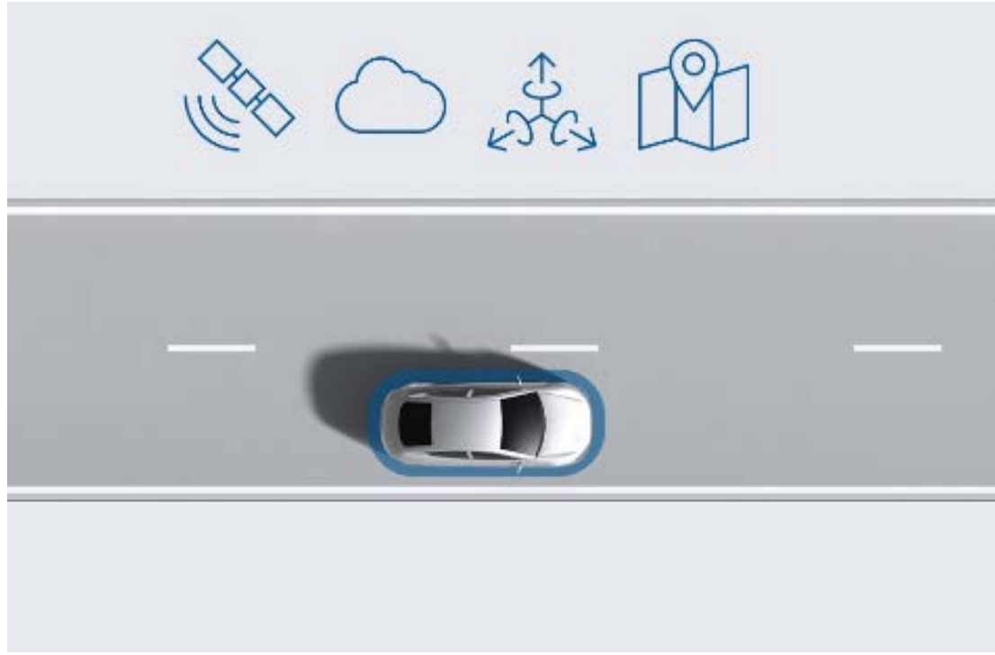
Accuracy of the Position determination using GPS, cloud data, inertial sensors and digital maps
